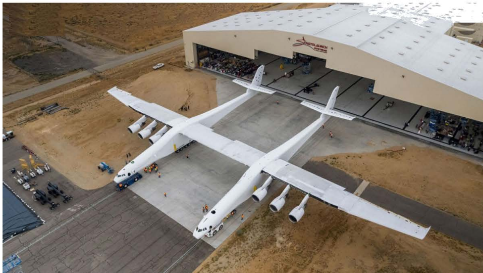
Designed and built by Scaled Composites, Stratolaunch is the largest composite-structure aircraft yet produced. Credit: Collier Research/Stratolaunch
