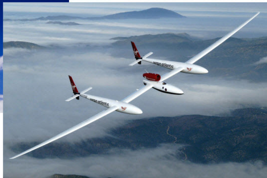
Figure 2. The long, slender wing of Steve Fossett's Global Flyer was designed to maximize lift and minimize drag. Similar aerodynamic principles apply to the structure of a wind turbine blade and can be used to guide design decisions.
