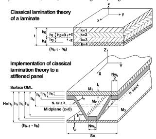
Fig. 3 Laminate formulation is extended to stiffened panels.
