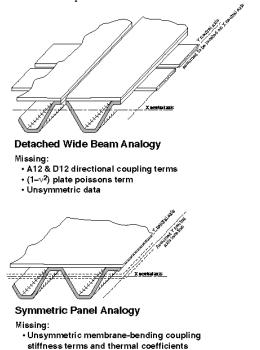
Fig. 2 Traditional formulation of stiffened panels using beam and plate analogies.
