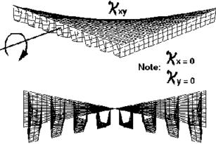
Fig. 11 Computed bending-twisting curvature of a 3-D FEM.
