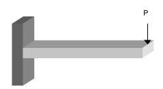
cantilevered beam with a vertical end load is to be designed using a rectangular cross section. The optimization problem is to minimize the weight of the beam while limiting vertical deflection and insuring structural integrity. In this case, the objective function is the weight. The obvious constraints on the problem are: 1) The stress,  $\sigma$  cannot exceed the material
