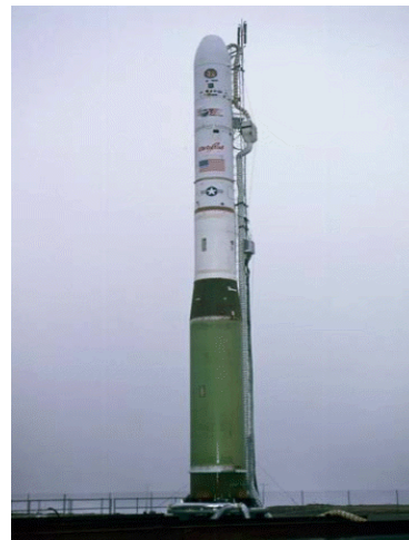
Fig. 4, Orbital's Minotaur OSP space launch vehicle with the existing honeycomb fairing.
