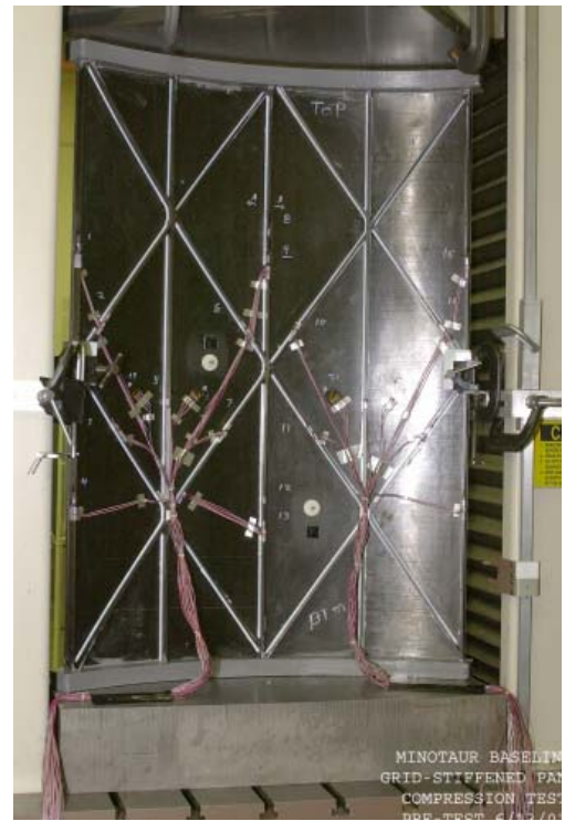
Fig. 9, Grid stiffened test panel in loading cell.
