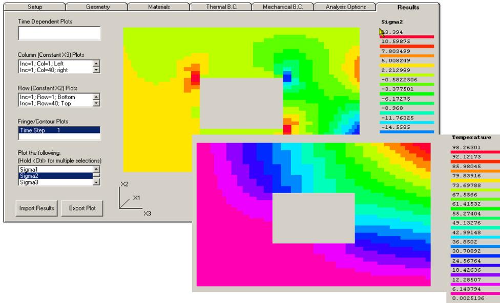
Figure 5: Results of the HOT-SMAC analysis are plotted on the **Results** tab. Contour (fringe) results available include temperature, stress components, plastic strain components, and displacement components. The **Results** tab also allows line plots of the solution.
