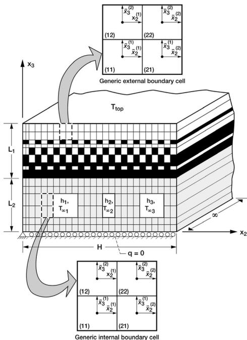
Figure 1: Example HOTFGM analysis geometry. The smoothing technique within the analytical formulation enables use of the rectangular subcell "mesh."
