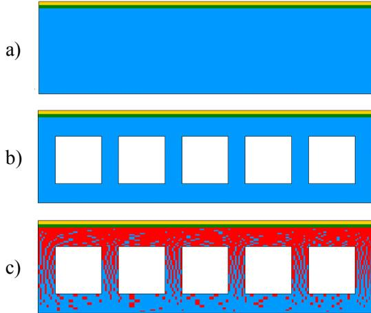
Figure 7: Panel configurations. a) no cooling channels, b) monolithic substrate, c) FG substrate
