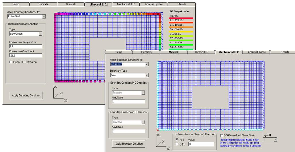
Figure 4: General or pre-defined thermal and mechanical boundary conditions are entered on the thermal B.C. and mechanical B.C. tabs, respectively.
