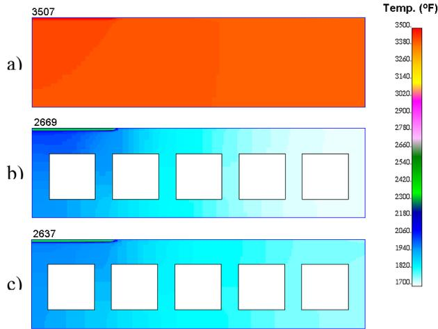
Figure 9: Temperature fields predicted in the plates predicted by HOT-SMAC. a) case 1, b) case 2, c) case 4.
