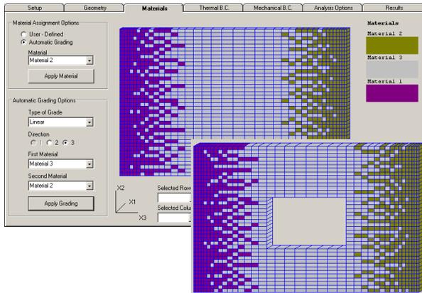
Figure 3: Material assignments for subcells are provided on the **Materials** tab. This tab also allows automatic uniform, linear, quadratic, or uniform grading of the materials, and specification of voids (i.e. windows).
