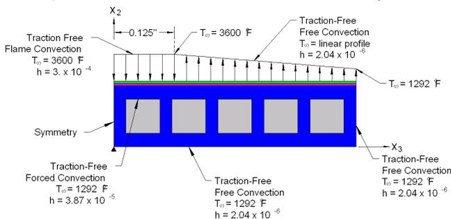
Figure 6: Cooled plate boundary conditions. Note: Symmetry is employed. Units for  $h$  are  $\text{BTU}/(\text{in}^2 \text{ s } ^\circ\text{F})$ .
