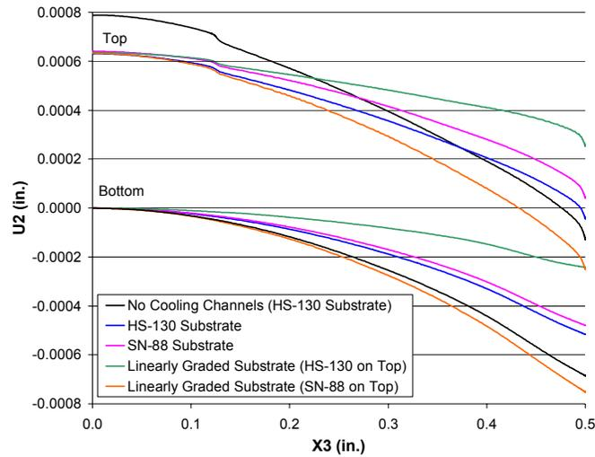
Figure 8: Vertical displacement along top and bottom of the plate predicted by HOT-SMAC.
