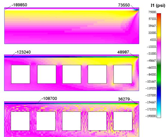
Figure 10:  $I_1$  stress invariant fields in the plates predicted by HOT-SMAC. ( $I_1 = \sigma_{11} + \sigma_{22} + \sigma_{33}$ ) a) case 1, b) case 2, c) case 4.
