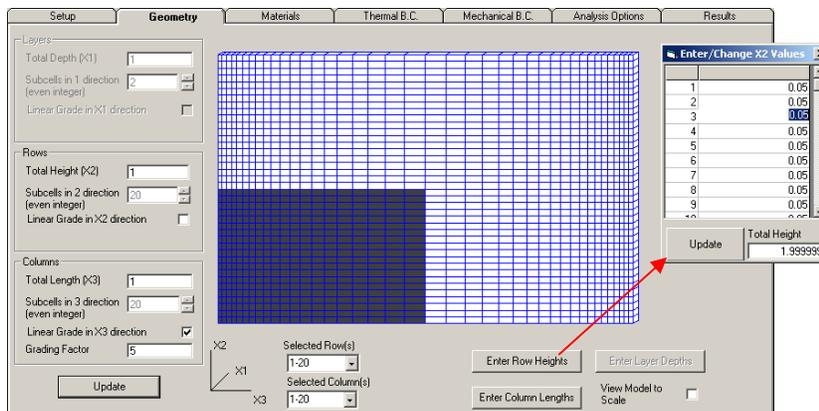
Figure 2: The **Geometry** tab allows specification of the problem dimensions, number of subcells, and the row heights and column widths
