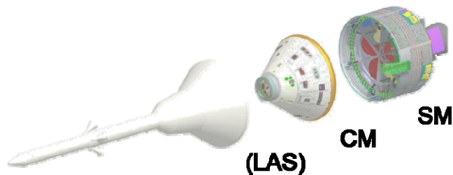
Fig.2, The Crew Module (CM) interfaces with the Service Module (SM) and the Launch Abort System (LAS).
