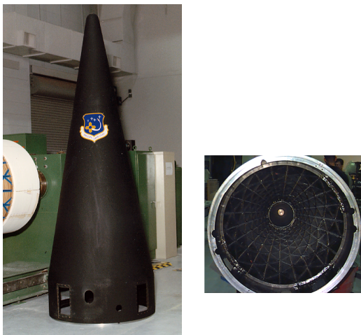
Figure 2. AFRL's AGS Fairing for BMDO's Combined Experiments Program (CEP), Side-View and End-View
