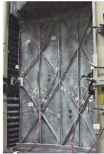
Figure 7. Boeing Stabilized Single Lap-Shear Test
