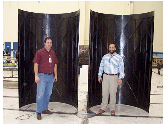
Figure 1. Advanced Grid Stiffened (AGS) Structure Configuration
