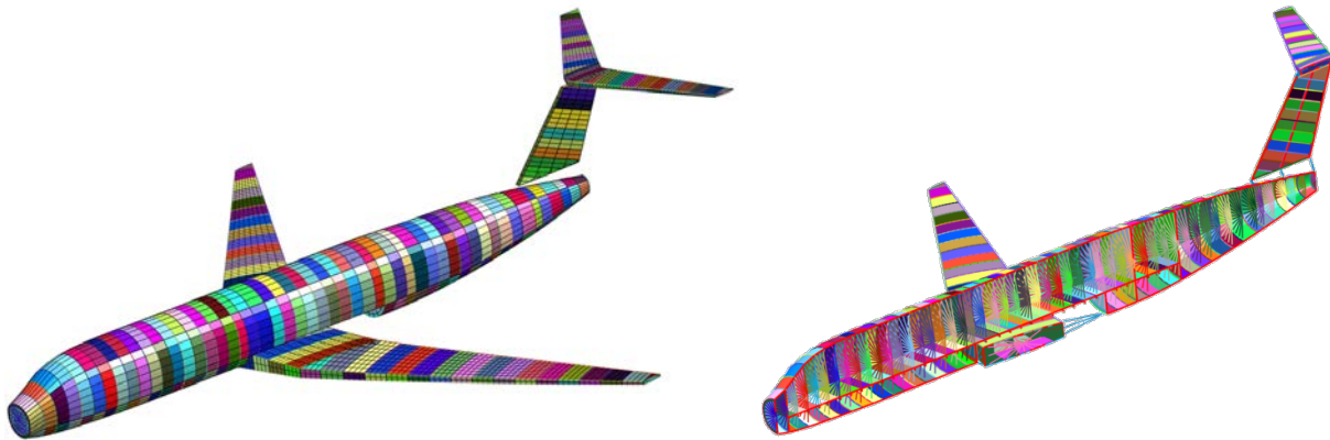
Figure 11. Global Structural Finite Element Model
