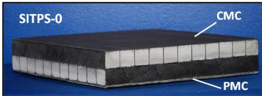
Figure 6. SITPS-0 test specimen, overall dimensions 292mm x 292mm x 57.15mm. 25.4 x 25.4 mm AETB-16 bars, wrapped with SiC fabric. PMC bottom facesheet bonded to panel.
