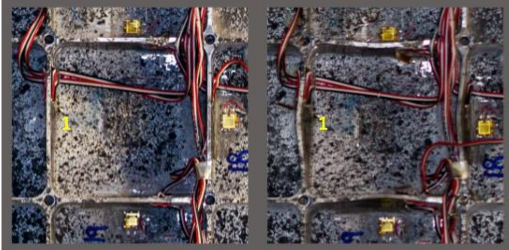
Figure 40: The inner-most webs before (left) and after (right) the inverted drop test.
