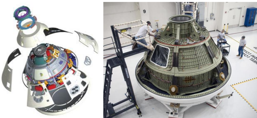
Figure 2. Orion Crew Module (CM). (Left) exploded view. (Right) As fabricated Orion Ground Test Vehicle (GTV) with baseline composite HSC structure attached.
