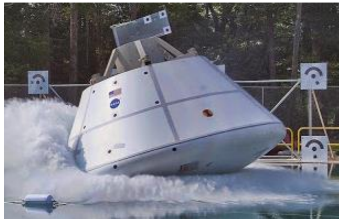
Figure 5. Orion boilerplate test article (BTA) splashing down in Langley's Hydro Basin.
