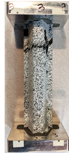
Fig. 5, Single stringer crippling test data from NIAR testing 2019 with low scatter and ultimate collapse load analysis prediction to within 4% of test average.
