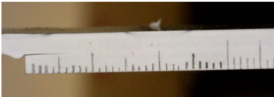
Fig. 13 Single Lap Joint with Embedded Crack, Showing Markings Used to Track Crack Growth
