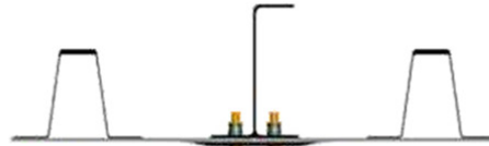
Fig. 23 - Hat Stiffened Panel Longitudinal Construction Joint Concepts
