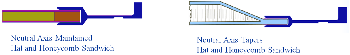
Fig. 24 - Common end frame geometry for sandwich and stiffened panels. (Left) the web of the metallic end frame is positioned over the neutral axis of the acreege panel to avoid load eccentricity caused from applying load off the neutral axis of the acreege panels. (Right) the acreege panel is tapered to a solid laminate then inserted into the metallic clevis joint.
