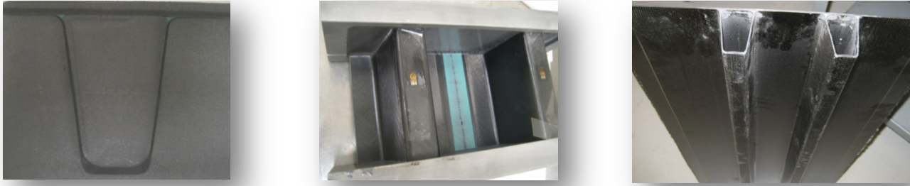
Fig. 7 - Fabricated hat panels; 2010 design
