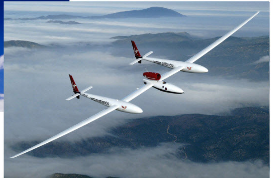
Figure 2. The long, slender wing of Steve Fossett's Global Flyer was designed to maximize lift and minimize drag. Similar aerodynamic principles apply to the structure of a wind turbine blade and can be used to guide design decisions.
