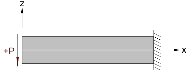
Fig. B.1. Positive sign convention for external shear loading on a beam.
