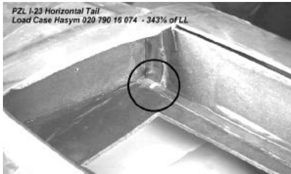
Fig. 8 View of the interior of the structure, after removing part of the skin.
