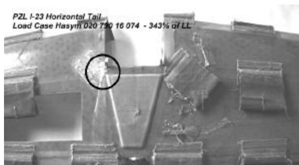
Fig. 7 Zone of initiation of failure - lower skin
