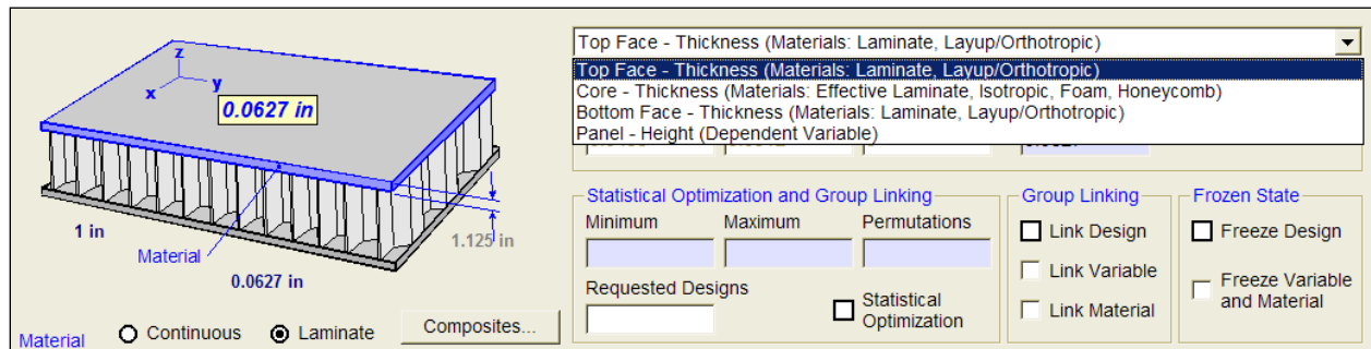
Fig. 7, Honeycomb Sandwich Panel Optimization Variables.
