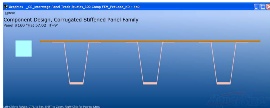
Fig. 18, Optimum Hat Stiffened Panel Scale Cross Section, Uniform Stiffener Dimensions
